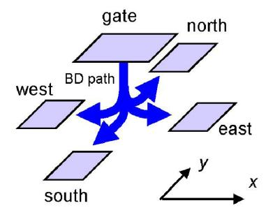
The electrons injected through the BD spot are collected by the four grounded contacts
