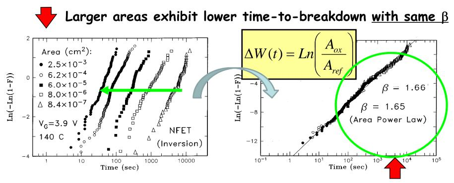
All curves can be merged into a single one by a vertical shift
