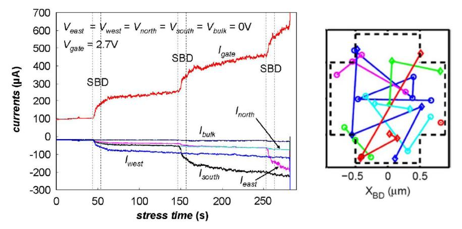
Current traces recorded during a constant voltage stress allow detecting the BD spots locations
