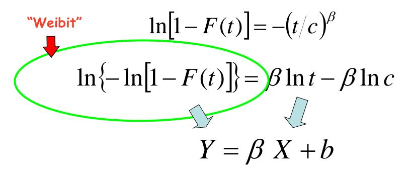
Weibull data are fitted by a straight line with slope  $\beta$
