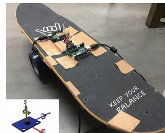
Prototype equipment (for torsion stiffness evaluation/ behavior monitoring)
