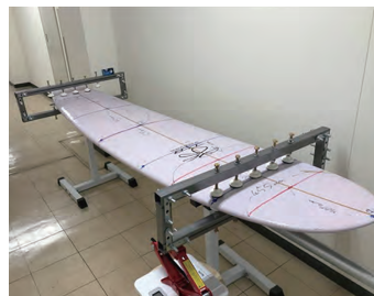
Prototype equipment (for torsion stiffness evaluation/ behavior monitoring)
