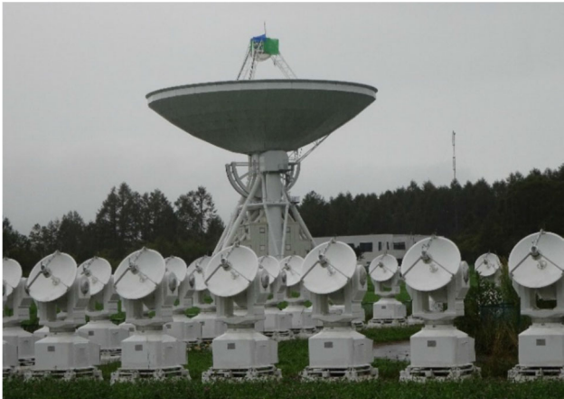
Fig.8 Simultaneous view of 45 meter Radio Telescope and a heliograph antenna array
