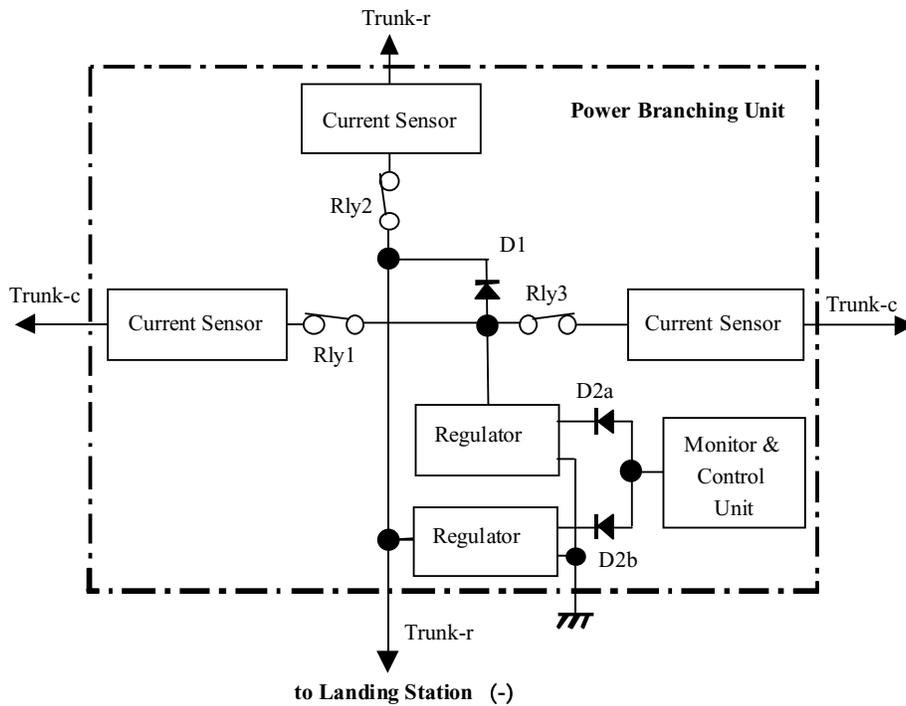
Figure 8 Proposed configuration of a power branching system in a PBU for CV power feeding system
