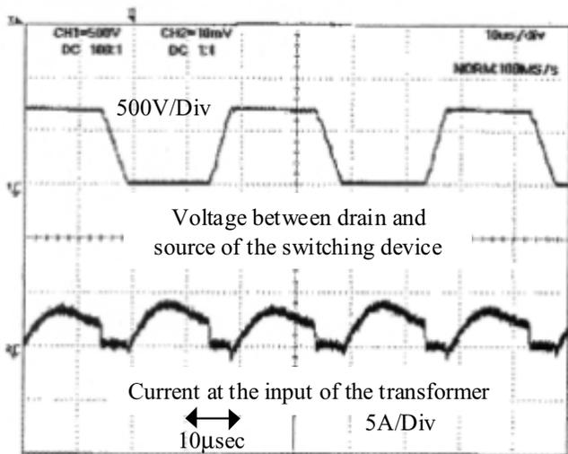
Figure 6 Observed waveform of the current to current converter
