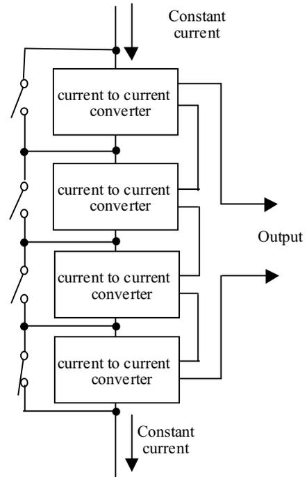
Figure 5 A typical configuration of a current source that will be placed in the PBU
