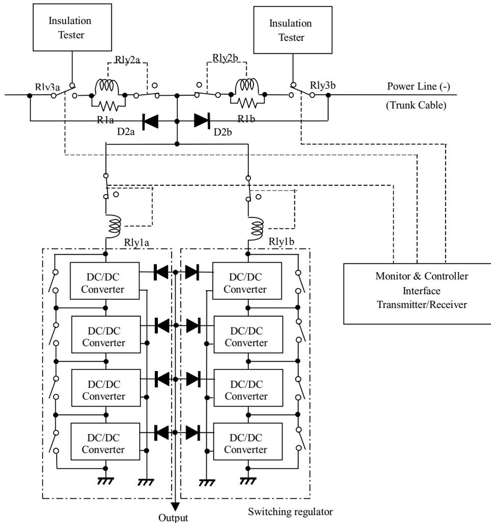
Figure 7 Proposed configuration of the underwater power source for each observation nodes
