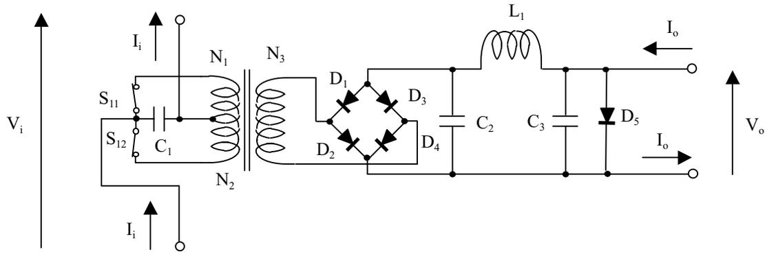
Figure 3 Basic circuit of the current to current converter
