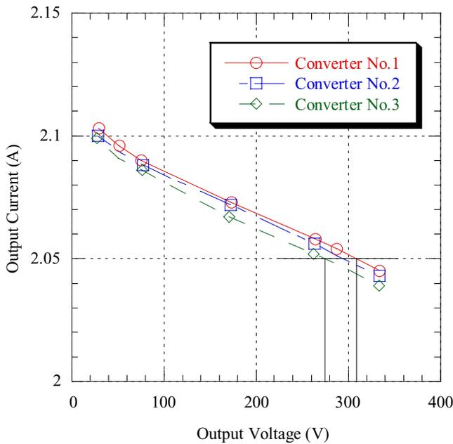
Figure 4 The output characteristics of three prototype of the current to current converter
