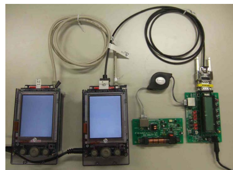
Figure 4. Experimental system to verify the operation of the SNTP server and the SNTP client
