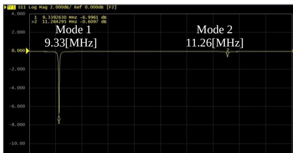
Fig.4 Resonant frequency of paired-spiral with PP winding direction when s=4\text{cm}
