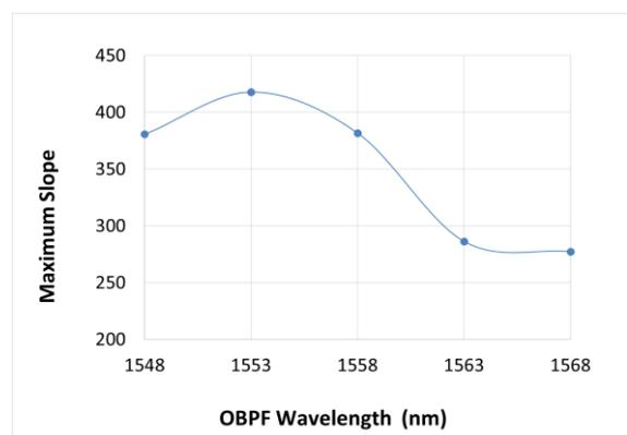
Fig. 4 Maximum slope as a function of OBPF wavelength
